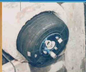
▪ Pipe stopper for leak testing
